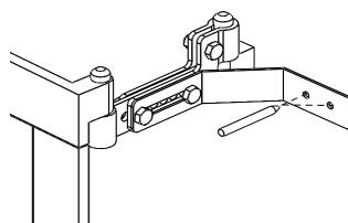
(UK) Drill two holes in the wall to fix the support bracket thus avoiding any lateral rotation.
